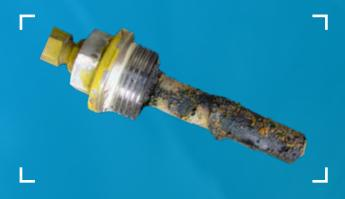
Clotted nozzles vapourise the odorant not sufficient anymore which leads to a higher consumption.
